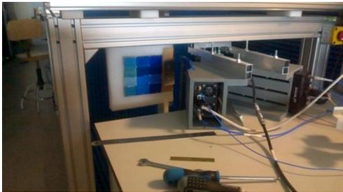
Fig. 2. Measurement of samples made of different pigments to obtain reference signals with the purpose of calibrating the equipment.
