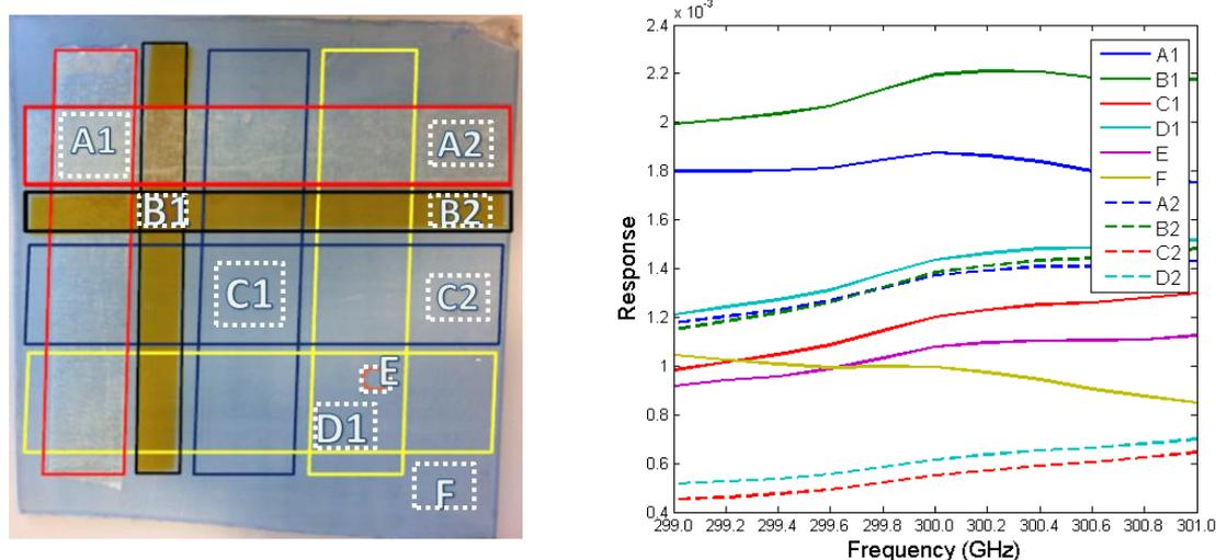
**Figure 2: (a) Defined patches and (b) the mean spectra plots for these patches.**
