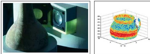
A **THz scanner for artwork analysis** has been developed, integrating novel graphene-based transmitters and receivers in the frequency bands between **140 and 330 GHz**. The THz radiation is focused on the surface under analysis through an **optical system**, enabling the **high-resolution automated scanning of real paintings and pottery** from museums.
